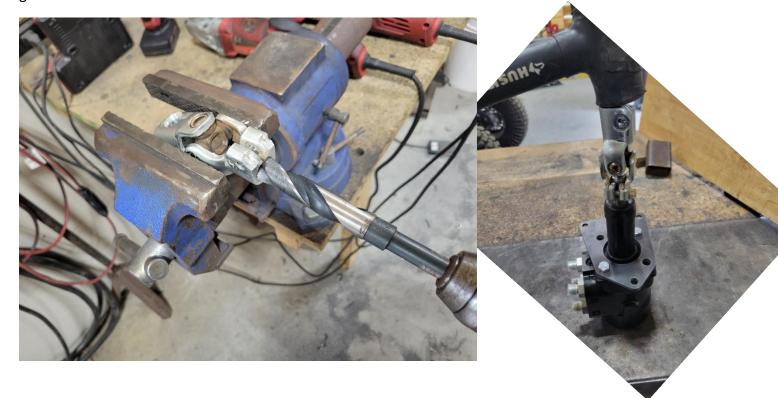
**Step 3.** Now assemble the Orbital valve in this order, steering column, bracket spacer, frame bracket. For now, leave the bolts hand tight. Install and tighten the 4 fittings into the Orbital valve at this time.
