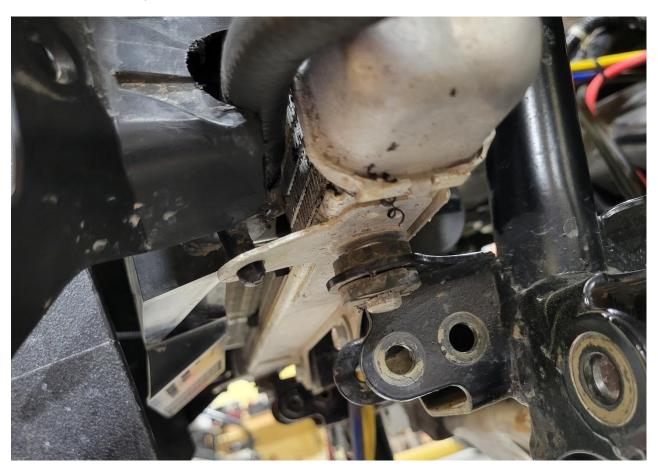
**Step 10.** The upper hose on the fluid cooler goes to the orbital valve and needs to be pushed on to the supplied hose barb and tightened down with supplied hose clamp. The lower hose goes up to the hydraulic pump return barb. This will be connected in a later step. (The pic below shows a 45\* fitting, but your kit may vary)
