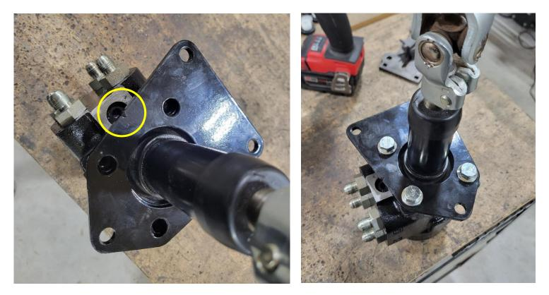
**Step 4.** Now install the Orbital valve assembly into the machine. Once you get the Orbital valve assembly in place, connect the yoke to the steering column before you start any of the frame bolts. Make sure to line up the yolk with the flat spot on the steering shaft so that the 10mm retaining bolt will install properly.
