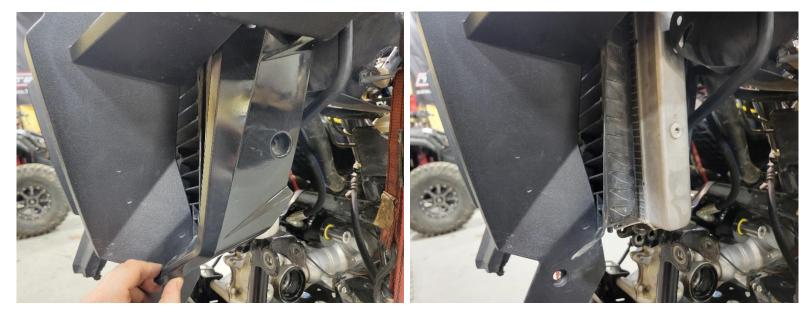
Step 2. Next push the lower grill pegs out of the radiator mounting holes on both sides as shown below.
