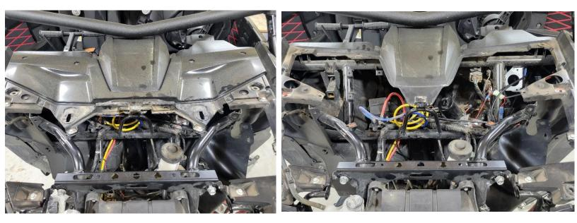
**Step 2.** Now that you have access to the EPS unit, remove the bolt that secures the steering yolk to EPS unit and the bolt that holds the yolk to the upper steering shaft. This will make it easier to remove the EPS Unit.
