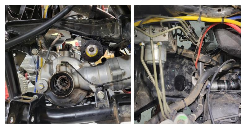
**Step 2.** Locate the 2 hydraulic lines that go from the ram to the orbital valve and install them. One end will have a 1/4" fitting for the ram side, and the other will have a 3/8" fitting for the orbital side.
