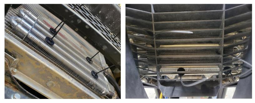
**Step 9.** Once the fluid cooler is secured and in place, put the radiator grill pins back into place, route the lines up to the orbital valve area, and reinstall the radiator side shroud.
