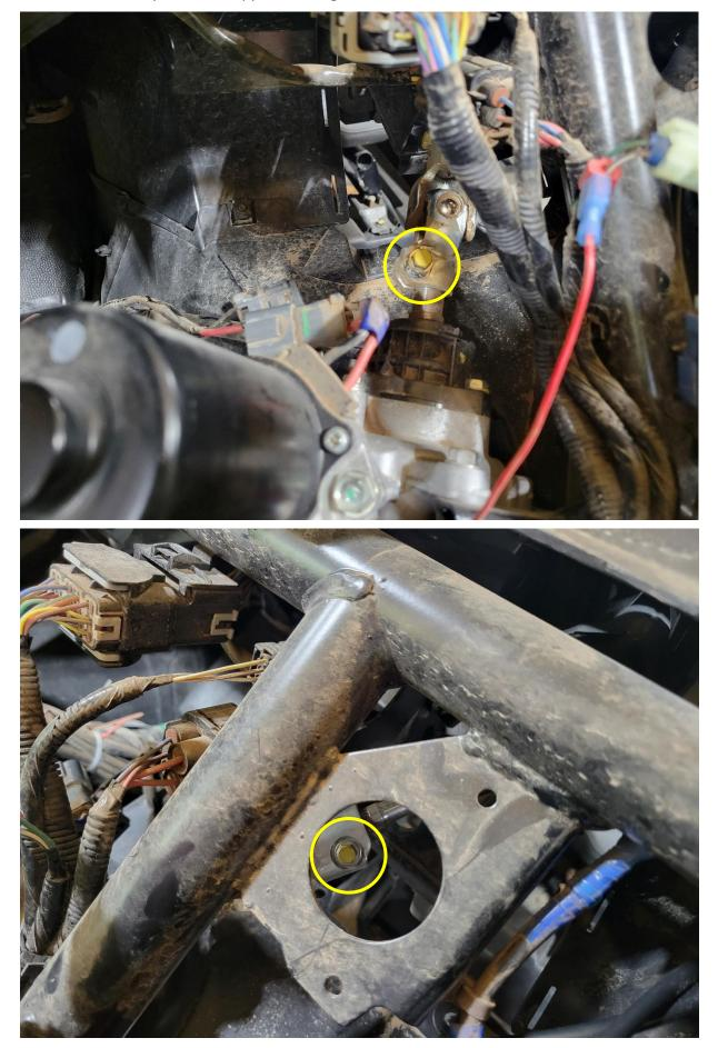
**Step 3.** Once you have removed the steering shaft bolts, disconnect the 2 electrical connectors from the EPS unit. Next remove the 3 bolts that mount the EPS unit to the frame, and remove the EPS unit from the machine along with the steering yolk.
