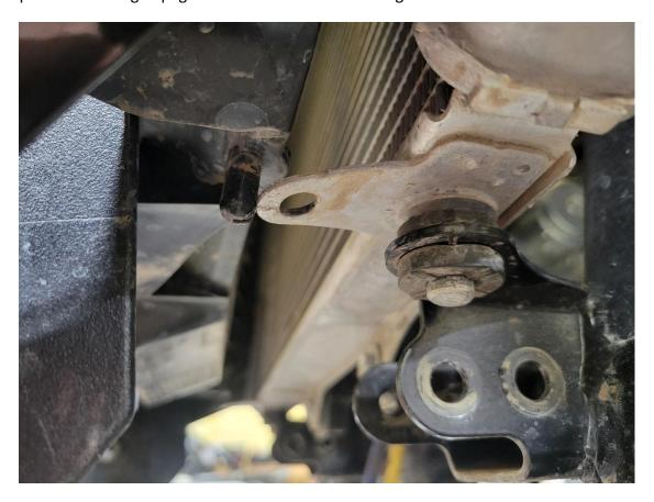
**Step 3.** Now locate the fluid cooler and use it to mark the radiator grill for trimming.
