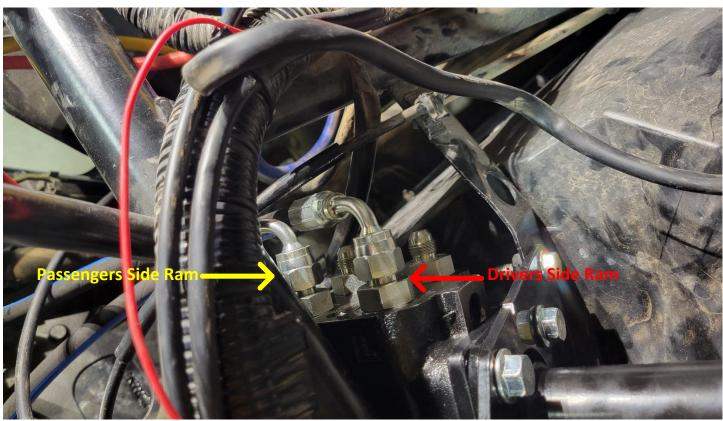
**Step 3.** Once each line is routed, tighten fittings down with a wrench on both the ram side and the orbital side.
