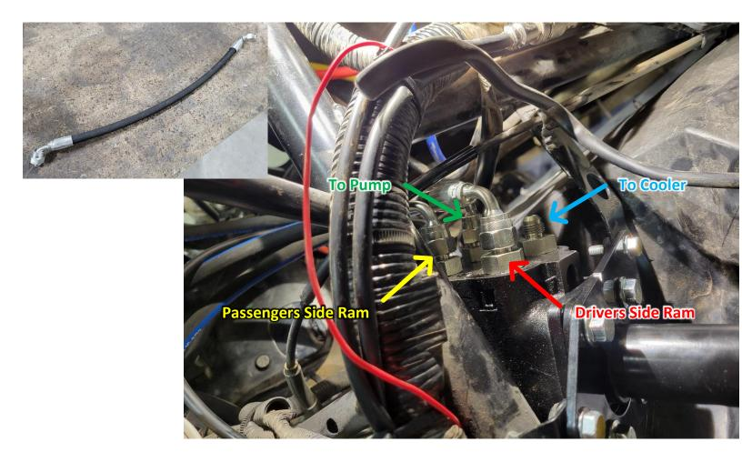
**Step 4.** Now, connect the lower low-pressure hose from the cooler to the return barb on the pump and secure with the supplied hose clamp. Also connect the high-pressure hose from the orbital to the pump and tighten.
