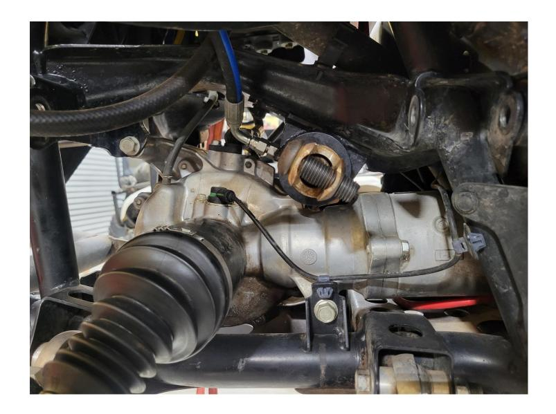
Ideally you want to line the clevis "ears" up with the hole in the hub assembly where the outer tie rod will attach. See pic below.
