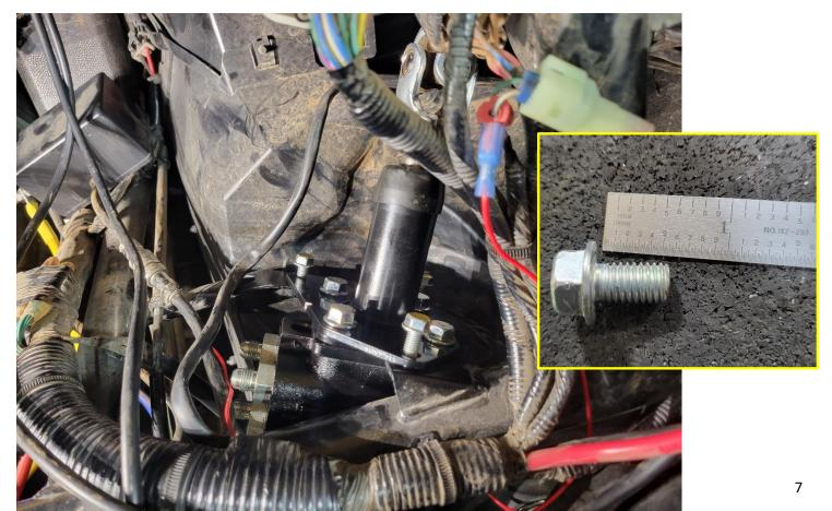
**Step 6.** Once everything is in place, tighten down the 3 bolts that secure the orbital valve bracket to the frame. Then tighten down the 4 bolts that hold the bracket and steering column to the orbital valve. **(Don't worry about whether your steering wheel is straight or not at this time)**
