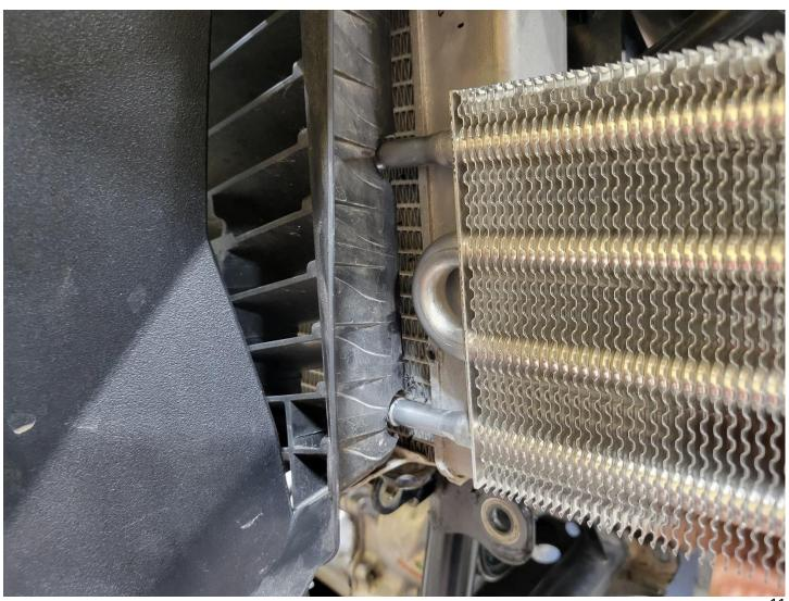
**Step 5.** Once the holes are trimmed, install the supplied hoses to the fluid cooler and put cooler into place for a test fit.
