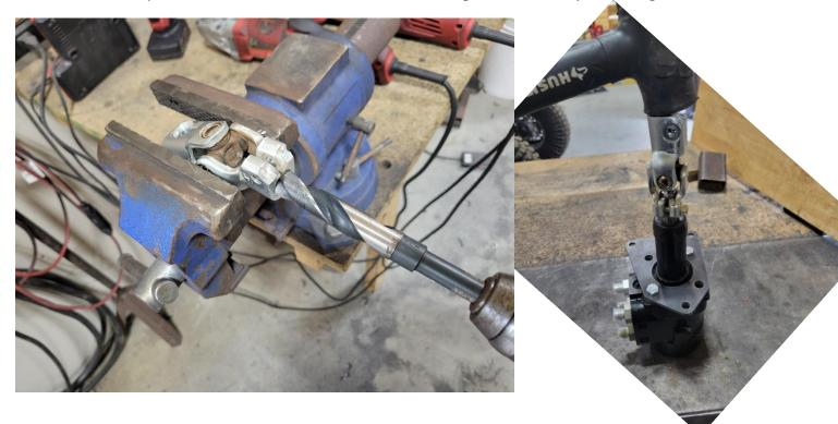
**Step 3.** Now assemble the Orbital valve in this order, steering column, bracket spacer, frame bracket. For now, leave the bolts hand tight. Install and tighten the 4 fittings into the Orbital valve at this time.
