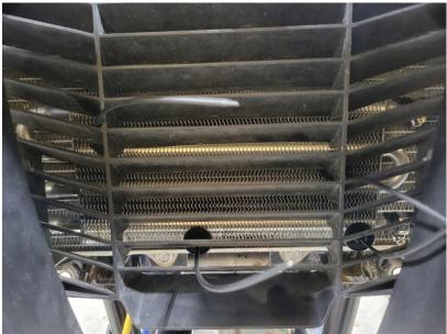
**Step 9.** Once the fluid cooler is secured and in place, put the radiator grill pins back into place, route the lines up to the orbital valve area, and reinstall the radiator side shroud.
