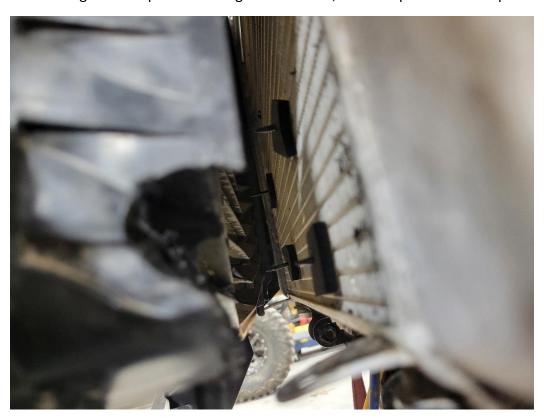
**Step 8.** Slide the cooler into place and feed the "EZ mount rods" through the cooler. Once in place, slide on the flat plastic holding washers, followed by the tiny locking cones that lock the washers into place and hold everything together. (See pic below) Trim the excess rods.
